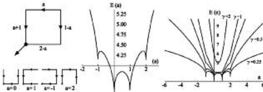
Figure 7. The 4-bond lattice. (Top left) the 4-node arrangement, with indications on the currents that respect continuity (note that a unit flux is injected at each node); (bottom left) the only for possible trees correspond to the cases  $a=0, -1, 1, 2$ . (Center) The energy function  $E(a)$  vs.  $a$ ; (Right) Energy functions  $E(a)$  vs.  $a$  for the cases  $\gamma=0.5, 0.75, 1, 2$  (after Banavar *et al.*, 2001).
