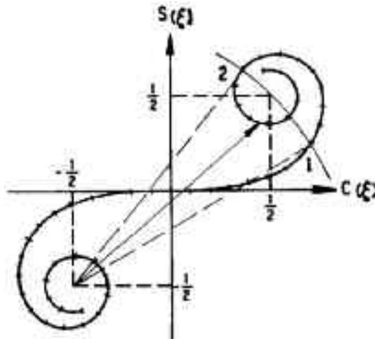
Fig. 2. Cornu spiral [8]. The value of  $\xi$  is marked along the curve while the values of the Fresnel integrals  $C(\xi)$  and  $S(\xi)$  are given along the abscissa and ordinate, respectively. One-half of the square of the magnitude of the vector from the point  $(-\frac{1}{2}, -\frac{1}{2})$  to a point on the curve with given  $\xi$  gives the probability density for that value of  $\xi$ .
