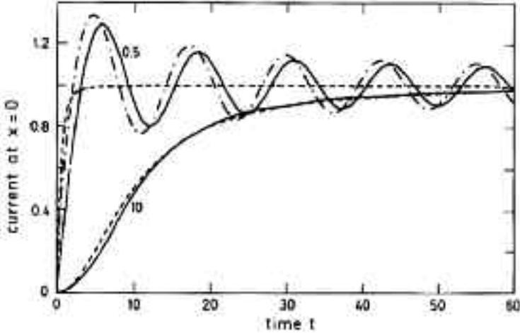
Fig. 5. Tunnelling current (in units of  $\hbar k/m$ ) as a function of time (in units of  $\hbar m/(\hbar k)^2$ ) for slow ( $\varepsilon=10$ ) and fast ( $\varepsilon=0.5$ ) lowering of the zero-range tunnelling barrier. The exact results (full lines) are compared with the current derived from the sudden limit (dash-dotted line). M. Kleber, *Physics Report* 236 (6) 1994 p. 384[9].
